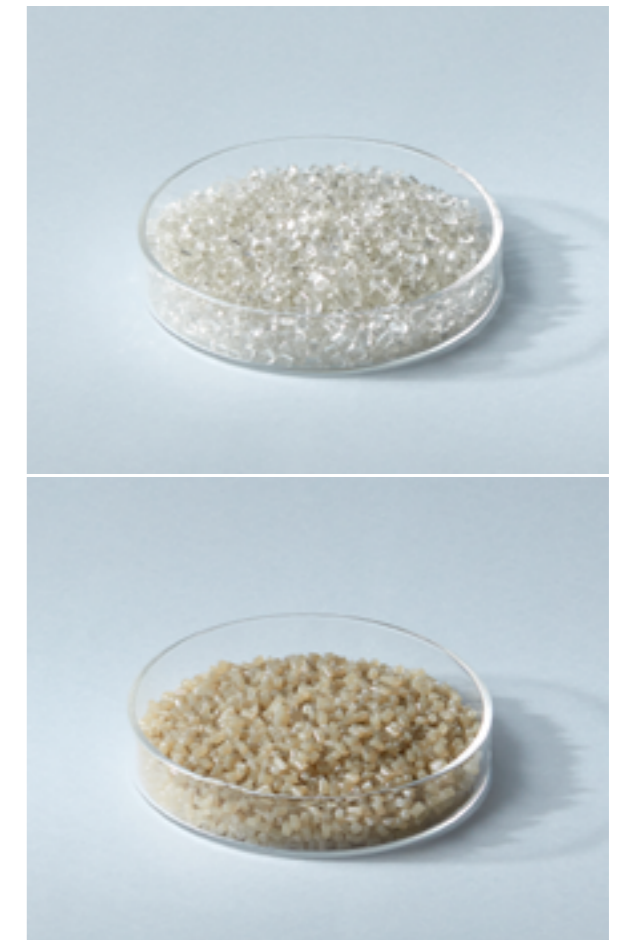
OBP PET & PA pellets from ocean waste PET bottles, fishing nets
