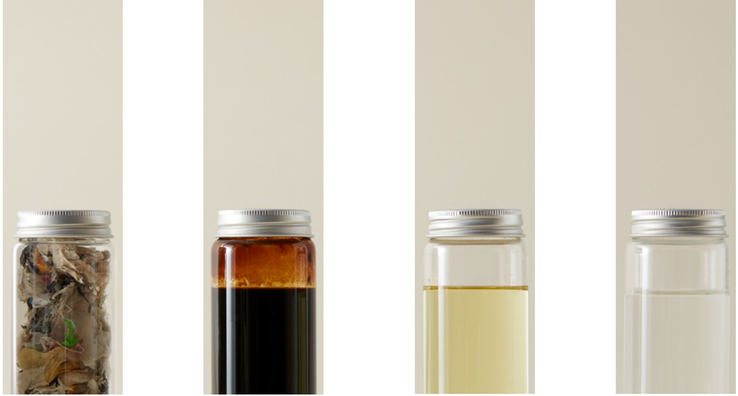
Circular Pyrolysis Oil' and 'Refined Pyrolysis Oil' from chemically recycled waste plastics
